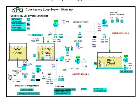
Good stock consistency control is accepted as a cornerstone of a low variability operation. In spite of its importance, there are often many problems found with the design and operation consistency loops. Common problems include inadequate mixing in stock chests. inappropriate sensor selection, dilution header pressure control. unnecessarily slow consistency controller tuning, consistency poor sensor calibration, poor management of consistency setpoints
