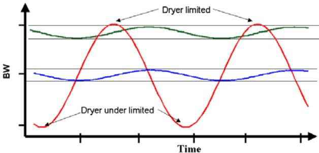
Cyclic variability often results in the over application of chemicals, energy or high-cost fibre. Reducing cyclic variability can therefore decrease *operating costs*, whether the variability originates in the raw material process source (i.e. chemical flow variability, steam pressure variability) or from an external process disturbance that is causing product variability.
