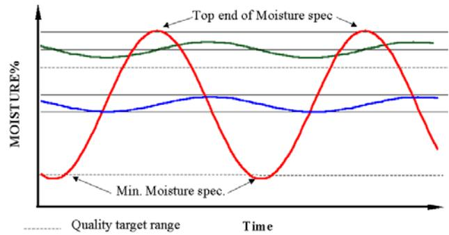
In the example below, reducing the ClO2 variability from the red line to the blue line will allow the operator to target shift the ClO2 dosage (to the green line) while still achieving the brightness target.
