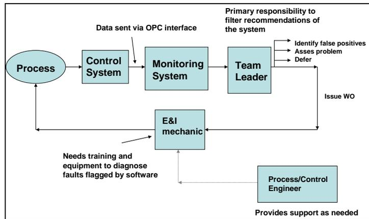
Figure 10 – shows a realistic view of the workflow using a Loop Monitoring system
