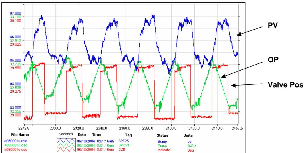
Figure 2 – Process variability caused by stiction
