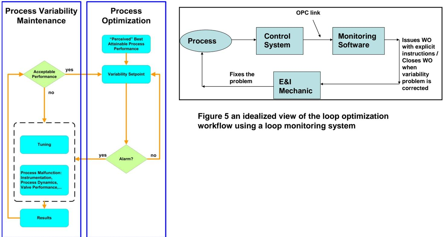
Figure 5 an idealized view of the loop optimization workflow using a loop monitoring system
