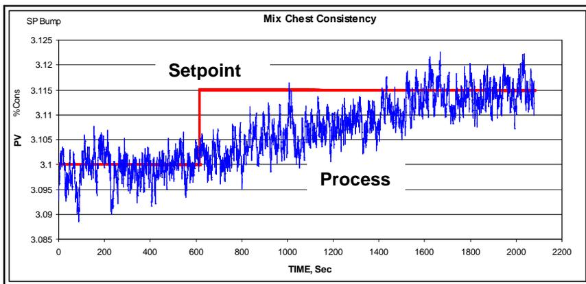
Figure 3 – Unnecessarily slow tuning on a consistency loop
