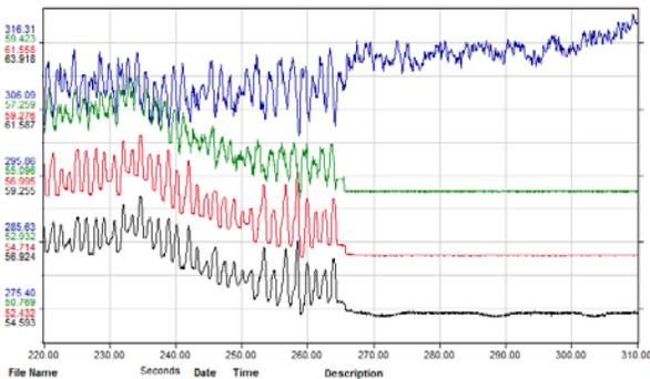
**Example 3 – Pressure, controller output and valve position are all cycling in Auto mode. The cycling stops in manual mode**
