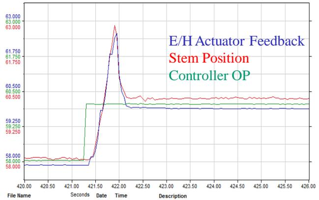
**Example 2 shows a valve with almost 100% overshoot of the steady state position.**
