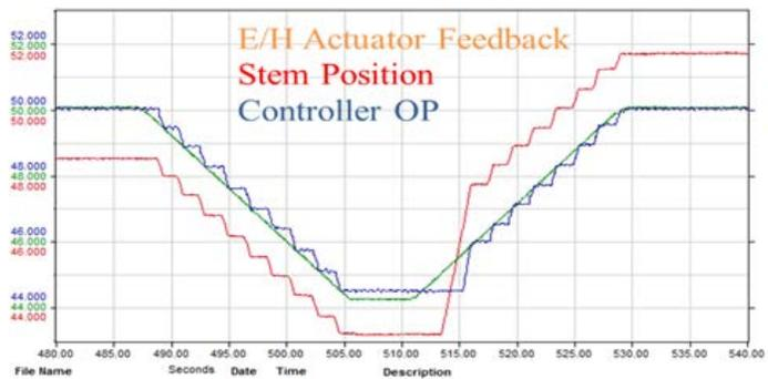
**Example 3b – Open loop step tests shows excessive valve step on output reversal**
