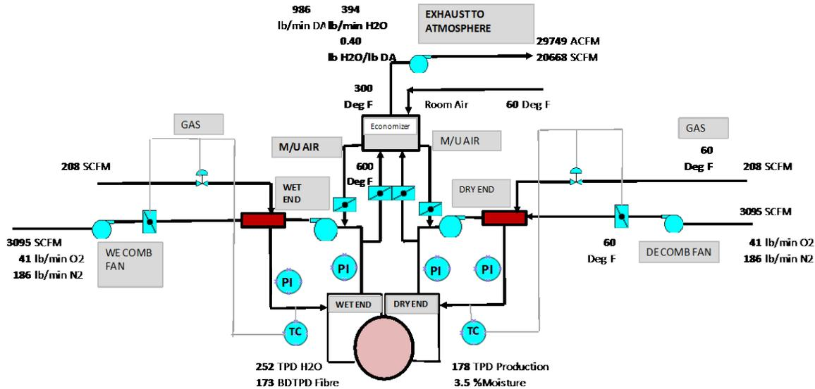
Figure 4 AirCap Flow / Energy Balance at 0.4 lb water per lb dry air
