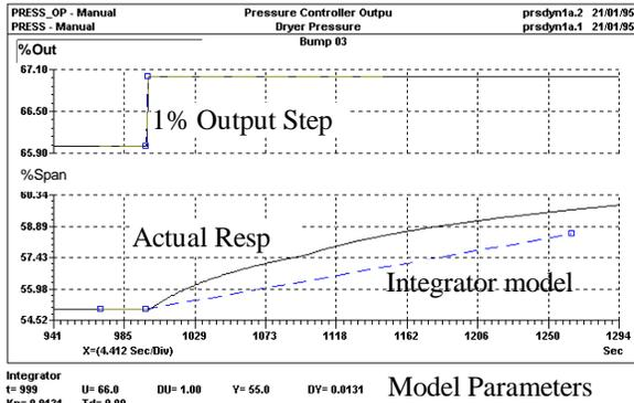
**Figure 10 Representing the Pressure Response as an Integrator**
