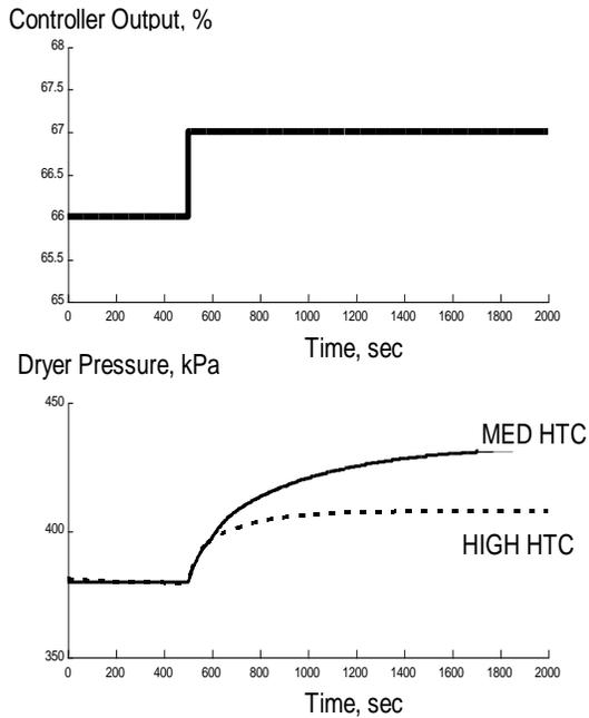
**Figure 3 Pressure Response to a Controller Output Step**
