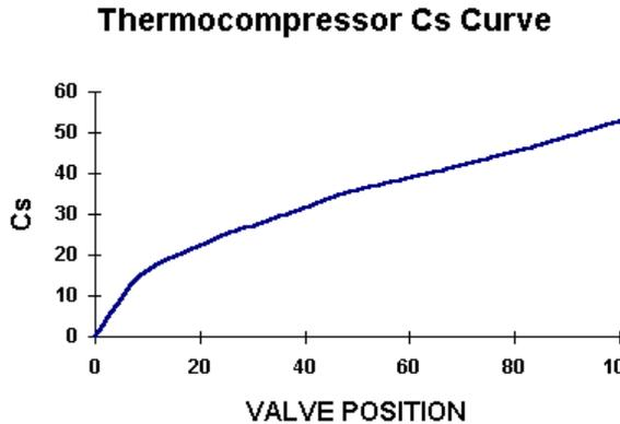
Figure 7 TC Flow Versus Valve Position
