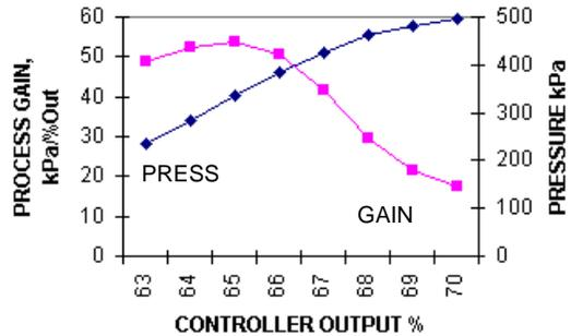
**Figure 6 Process Gain Versus Dryer Pressure**
