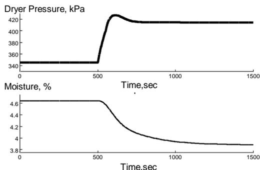
**Figure 2 Moisture Response To A Pressure Setpoint Step**
