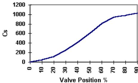
**Figure 4 Makeup Steam Valve Cs Curve**
