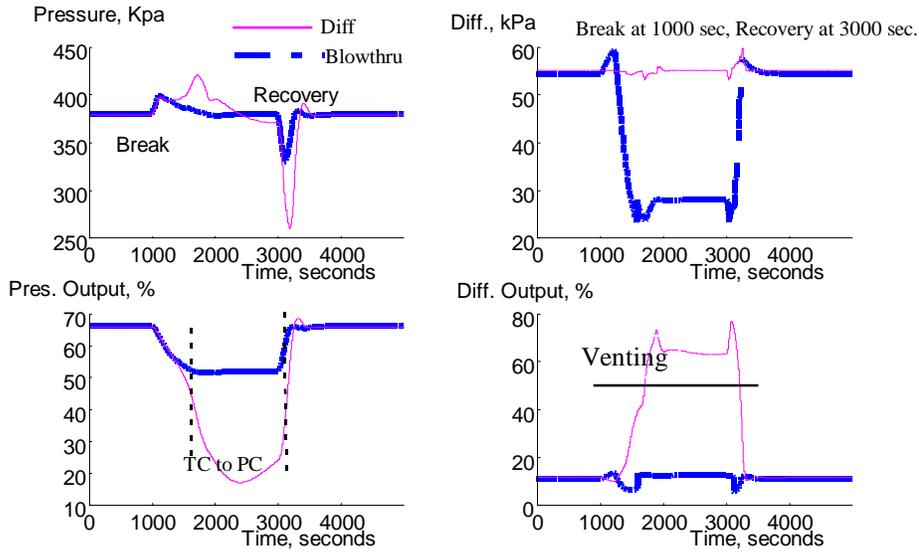
**Figure 9 Blow-through Versus Differential Control Response to Sheet Break/Recovery**
