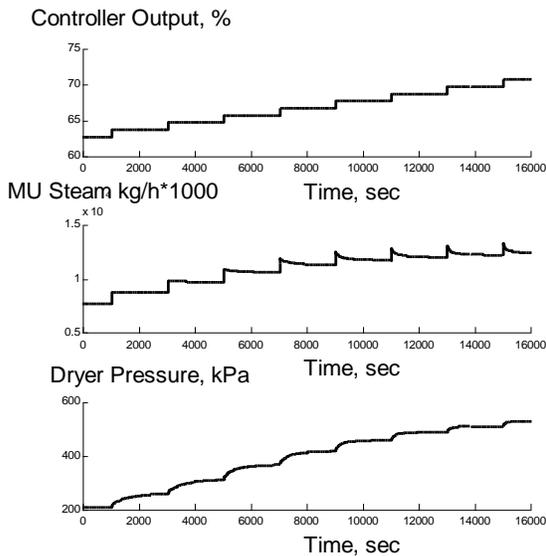
**Figure 5 Pressure And Makeup Steam Flow Response To Controller Output Steps**
