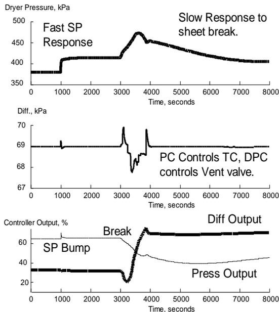
**Figure 11 Near-Integrating Tuning - Response to Setpoint Change and Sheet Break**
