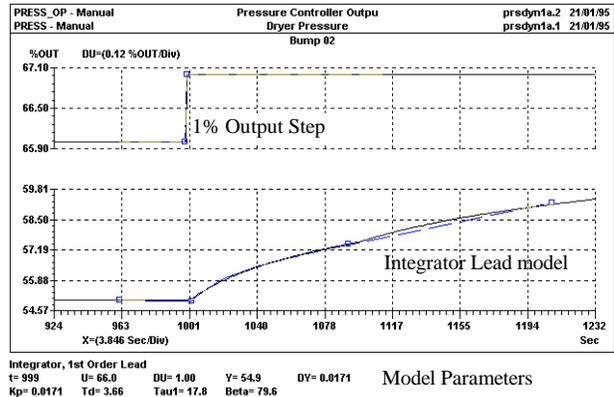
**Figure 12 Modeling the Response as Integrator Lead**
