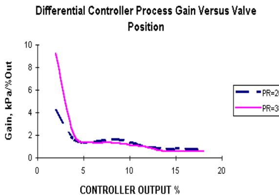
Figure 8 Differential Controller Gain Versus Operating Point
